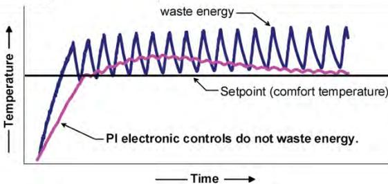
*Fig.2 - On-Off mechanical control vs. PI electronic control.*
